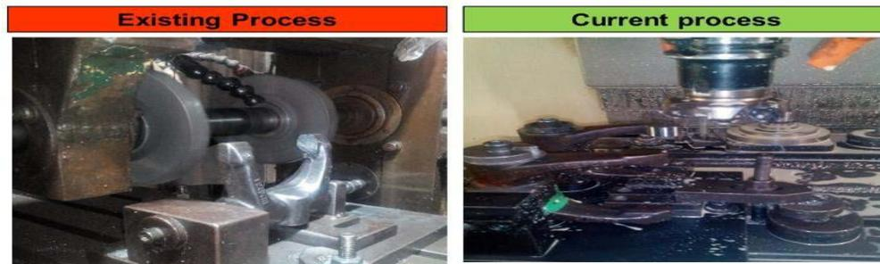
Conventional outside milling process to replaced with VMC Facing process to achieve consistency on pad thickness
