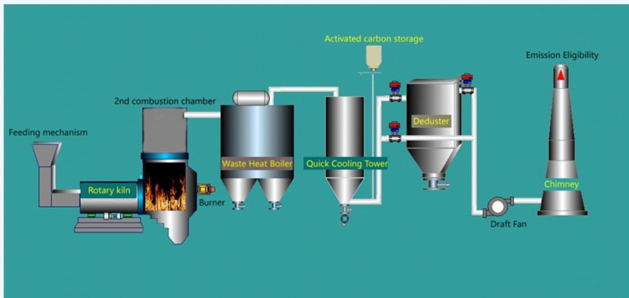
Figure – 7.2.3: Incineration Flow Diagram
