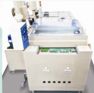
<Fortune One>: Automatic Gold stripping line
